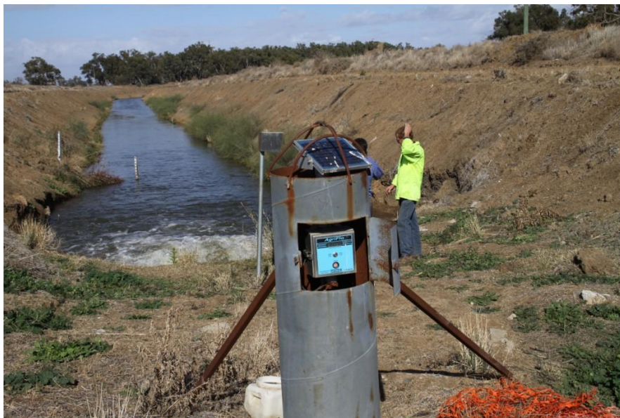
Figure 7 – Albert Priest Channel and regulator flow meter
